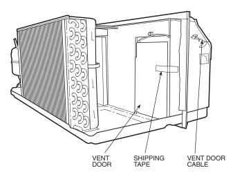
FIGURE 7 — LOCATION OF SHIPPING TAPE ON VENT DOOR
